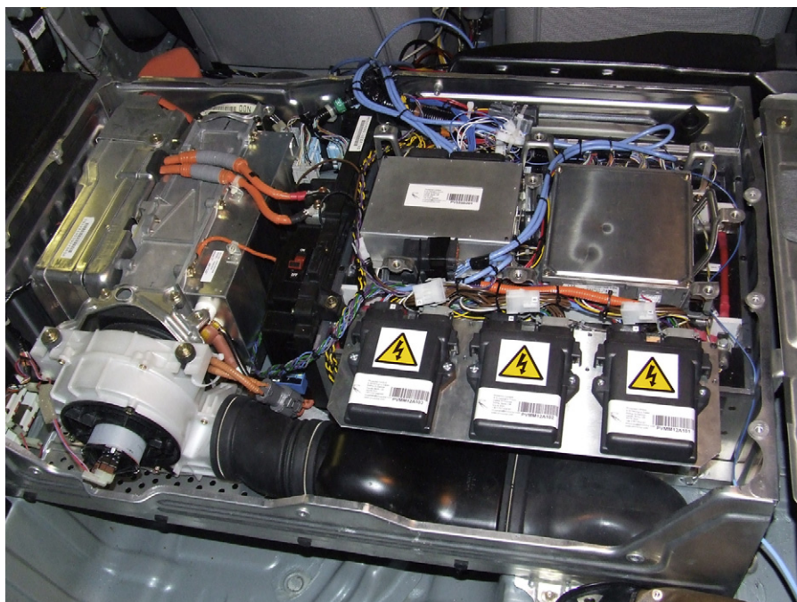
Fig. 4. The UltraBattery in place.
